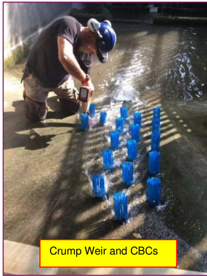
Figure 5.8 Option 7: Cylindrical Bristle Clusters on West or East Weir
